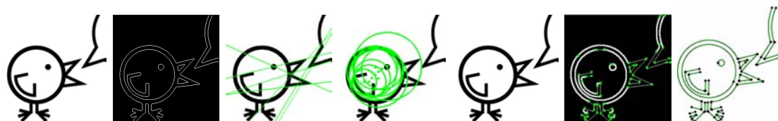
Figure 4.20: More complex combination of geometrical features. From left to right: original image, edge map, Hline, RHTcircle, RHTellipse, Etemadi, ELSD.
