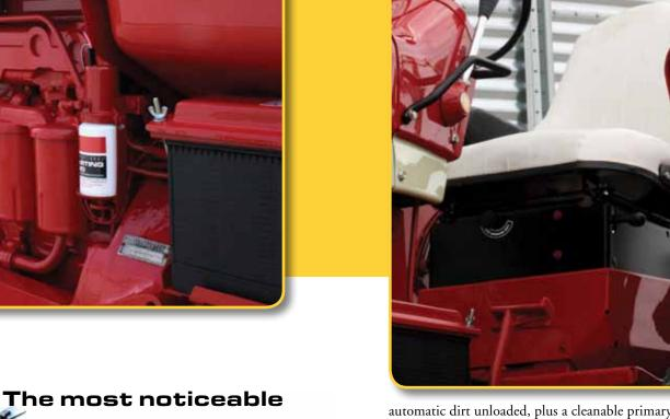
automatic dirt unloaded, plus a cleanable primary filter element. A secondary (inner) air cleaner element kept dirt out of the engine with 99.9% efficiency. A dash-mounted electric filter indicator tells you when the filters need to be serviced. A straight exhaust pipe was standard equipment on the 1256, however many farmers opted to install an oval muffler to quiet the turbo whine
