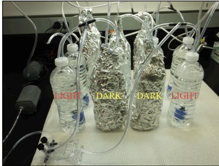
Figure 2 . General setup of a 4-bottle bioreactor system, varying only light regime(24:24 h, light:dark) across reactors.
