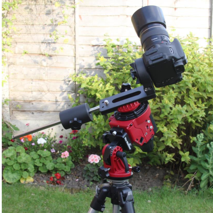
Figure 16 – A very portable imaging setup. This is a Sky Watcher Star Adventurer mount but other equivalent types are available.
