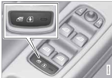
Control panel driver's door.
