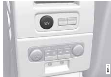
12 V socket in tunnel console, rear seat.
