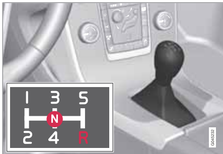
Gearshift pattern 5-speed gearbox.
