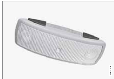
Rear roof lighting.
