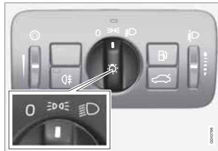
Headlamp control in position for position/parking lamps.
