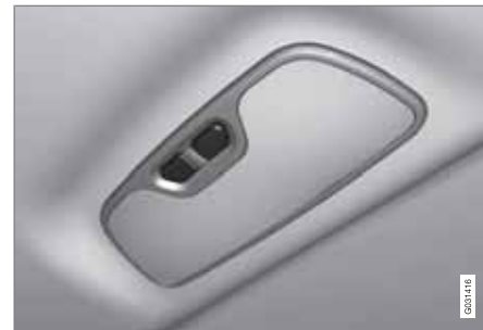
Rear roof lighting in cars with panorama roof.
