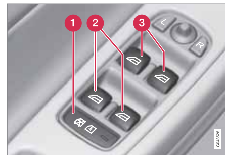
Driver's door control panel.
