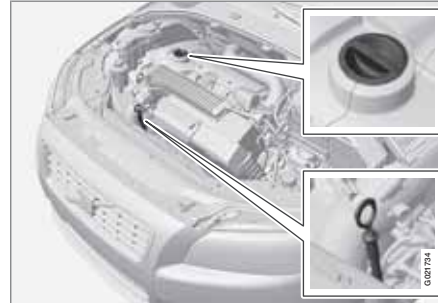
Dipstick and filler pipe.
