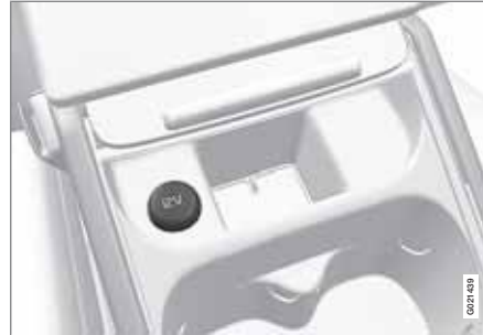
12 V socket in tunnel console, front seat.
