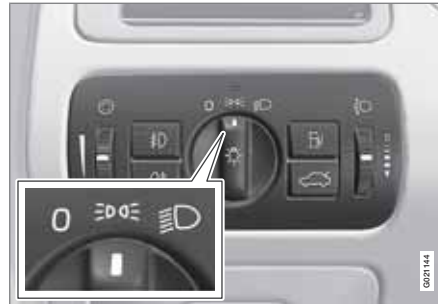
Headlamp control in position for position/parking lamps.
