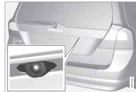
Camera location next to the opening handle.
