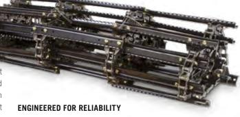
**Secure chain pin:** When it comes to proper tension in feeder chains, chain pins are key to holding everything together. Without proper tension, a stretched chain will jump off the gear – causing damage to the combine. Test results show that competitor feeder chain pins push off with half as much effort as our pins, causing their chains to stretch or break.
