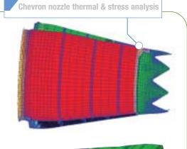
aerodynamic loads. The structure would have to be designed to ensure full life. Extensive testing both on an engine in a test cell, as well as fully instrumented flight testing, allowed GAG to correlate a detailed finite element model of the chevron nozzle. This model was then used to demonstrate full life capability at all the extremes of the operating envelope of the aircraft.
