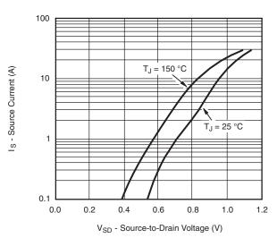
Figure 8 oure-Drain Diode Forward Voltage
