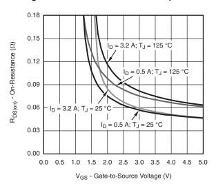
Figure 9 On Resistance VS. Gate-to-Source Voltage
