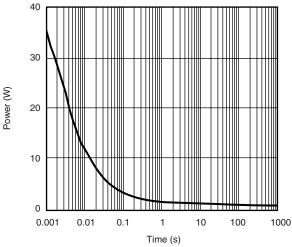
Figure 11 Single Pulse Power, Junction-to-Ambient
