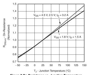
Figure 7 On-Resistance vs. Junction Temperature
