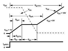
Figure 18. Gate Charge Waveforms
