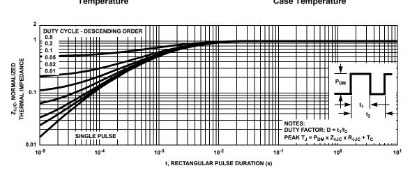
Figure 3. Normalized Maximum Transient Thermal Impedance
