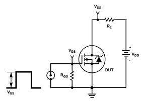
Figure 19. Switching Time Test Circuit
