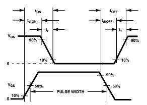
Figure 20. Switching Time Waveforms
