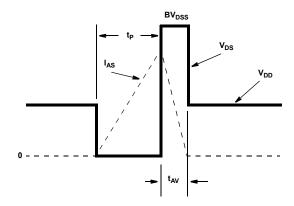
Figure 16. Unclamped Energy Waveforms
