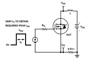
Figure 15. Unclamped Energy Test Circuit
