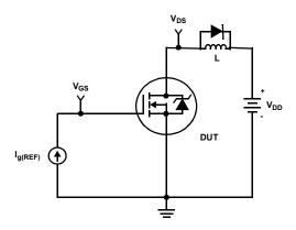
Figure 17. Gate Charge Test Circuit
