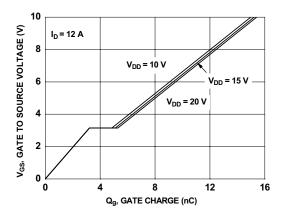
Figure 7. Gate Charge Characteristics
