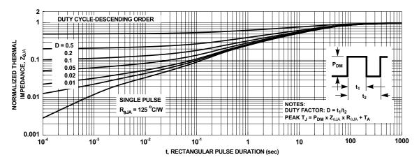
Figure 13. Junction-to-Ambient Transient Thermal Response Curve
