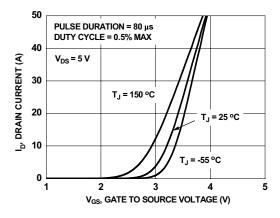
Figure 5. Transfer Characteristics
