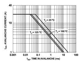
Figure 9. Unclamped Inductive Switching Capability
