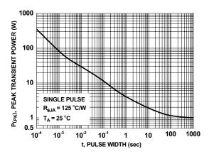
Figure 12. Single Pulse Maximum Power Dissipation
