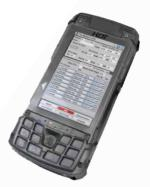
• Ruggedised Mortar Computer Internal GPS Touch screen Surveys calculation options Fire planning functions Ammunition stores
