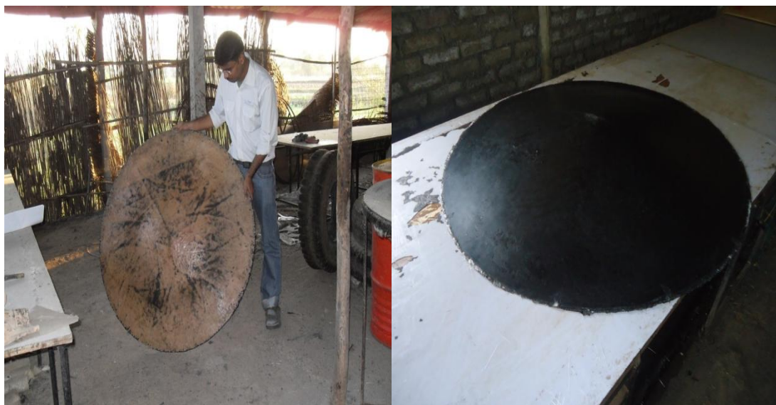
Figure 3.2: Mild steel dome and Fibre dome
