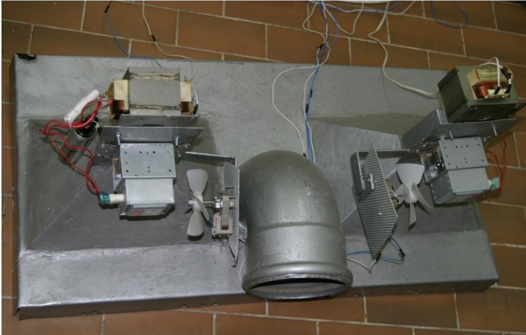
Figure 1: The twin microwave guns with Magnetrons and cooling fans.
