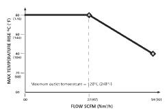
The inlet air temperature can be increased according to the above graph and the intelligent controller will hold any pre-set temperature irrespective of flow rate fluctuations.
