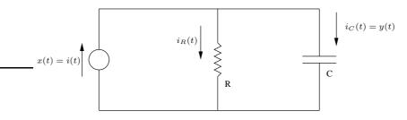
Suppose we are interested in the signal corresponding to the current through the capacitor as we change the current produced by the source. These are functions of time, and can be thought of as signals. In this case we can think of the circuit as a system: the input x(t) is the input current i(t), and the output y(t) is the capacitor current  $i_C(t)$ . The laws of physics (expressed as the theory of electrical circuits) let us find the output signal for any given input signal.
