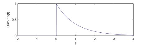
After the step the current initially all flows through the capacitor, which begins charging. Once charged, all the current flows through the resistor so the output signal goes to zero.
