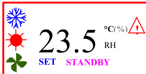
Figure 2-6 LCD of the interface module between Microface and the operator.
