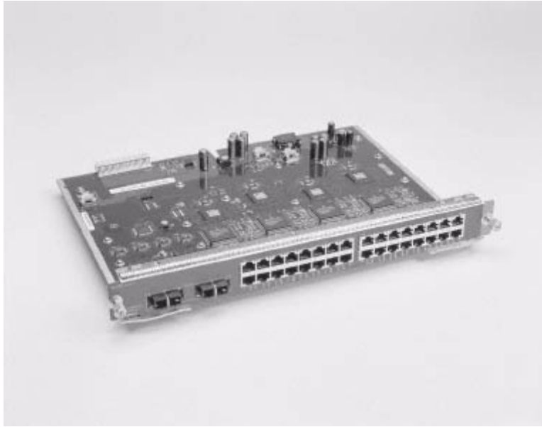
Figure 5-7 Catalyst 4000 series, 2-port Gigabit Ethernet, 32-port 10/100 line module
