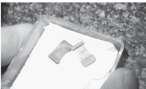
FIGURE 3. Metal components of the depressed collector
