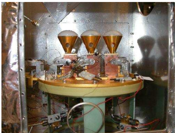
Figure 8: A photograph of three mixers installed in the JT cryostat before testing.
