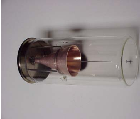
Fig. 2. First microwave photomixer using resonant laser-assisted field emission.
