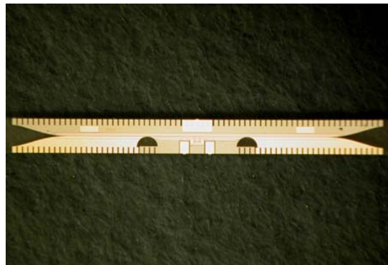
Figure 2: Superconducting chip containing two finline transitions, a beam combining directional coupler and two SIS tunnel junctions
