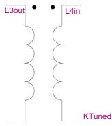
This device can be used to define coupling between inductors (transformers) or between transmission lines. This device also refers to a nonlinear magnetic core (CORE) model to include magnetic hysteresis effects in the behavior of a single inductor (winding), or in multiple coupled windings.
