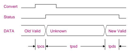
DATA refers to both the data and over-range signals. The Convert pulse can be any width, including zero. If the propagation delay between the rising edge of the Convert signal and the Status signal (tpsd) is zero, the data and over-range do not go to unknown but directly to the new value. There is a resistive load from <ref node> to <gnd node>, and from <in node> to <gnd node>, of 1/GMIN.
