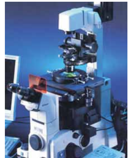
Figure 11. A continuous focus microscope (adopted from http://www.lin.com.tw/menu/products )
