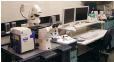
Figure 4. A setup of white laser confocal microscope. (adopted from http://www.lehigh.edu/~inbios/facilities/confocal.htm )
