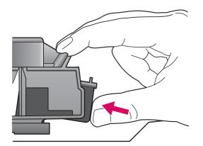
只有打开设备后,才能放入墨盒。 a 握住三色墨盒, 使 HP 标签朝上。 **b** 将三色盒放在左侧插槽的前方。 c 用力将墨盒推入该插槽中,将其紧紧卡住。 The device must be **On** before you can insert the print cartridges. **a** Hold the **tri-color** print cartridge with the HP label facing up. **b** Place the **tri-color** print cartridge in front of the **left** slot. c Push the cartridge firmly into the slot until it snaps into place. 放入黑色墨盒
