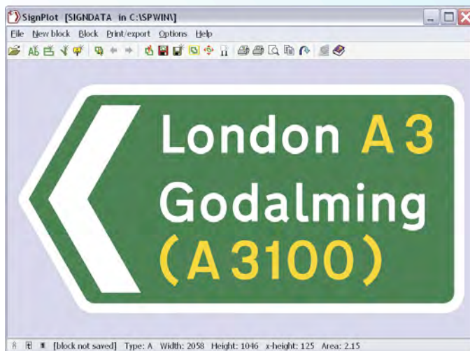
The weight and colour of the lettering is corrected automatically on the finished design.
