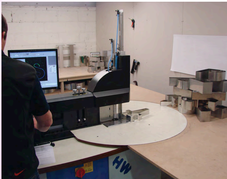
The bending machine is capable of producing built up letters in stainless steel.
